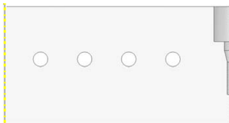
Type 1 has circular channels
